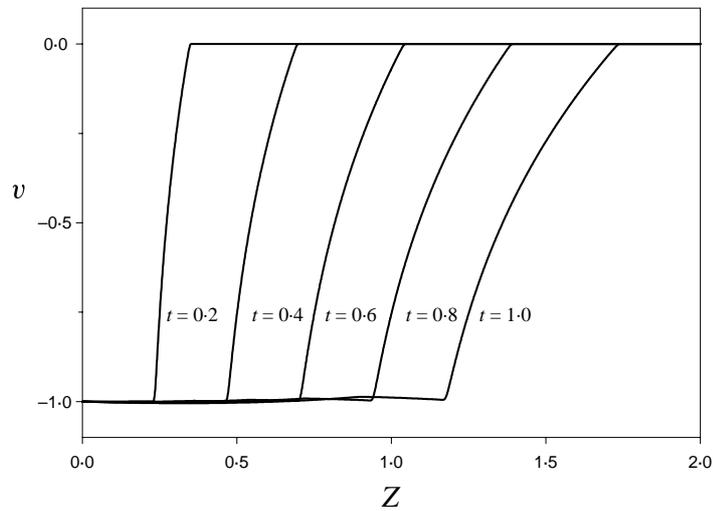
FIG. 9.  $v$  as a function of  $Z$  at various times for the Blatz–Ko model (2.28).  $L = 2$ ,  $v_0 = 1$ .
