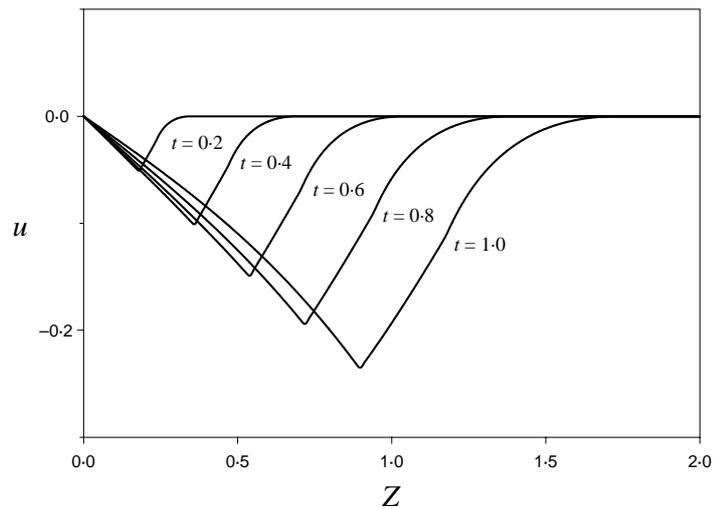
FIG. 10.  $u$  as a function of  $Z$  at various times for the Blatz–Ko model (2.28).  $L = 2$ ,  $v_0 = 1$ .
