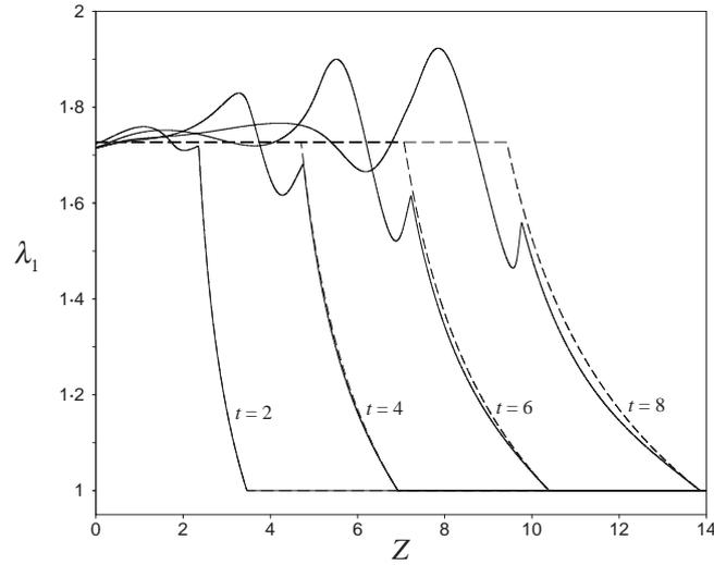
FIG. 11.  $\lambda_1$  as a function of  $Z$  at various times for the Blatz–Ko model (2.28). The dashed lines represent the simplified solution obtained from the limiting case.  $L = 14$ ,  $v_0 = 1$ .
