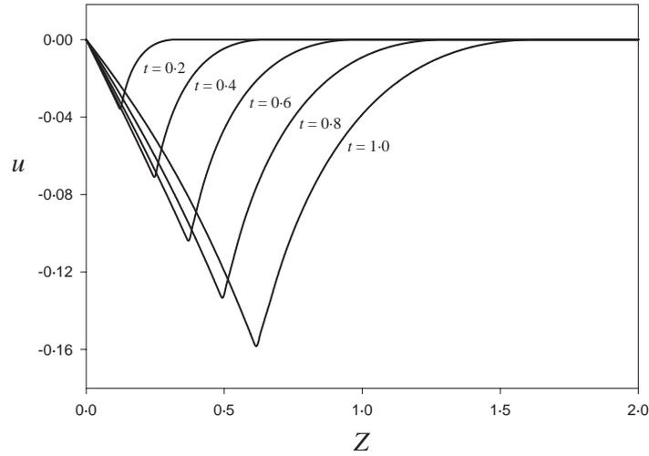
FIG. 4.  $u$  as a function of  $Z$  at various times for the Blatz–Ko model (2.19).  $L = 2$ ,  $v_0 = 0.5$ .
