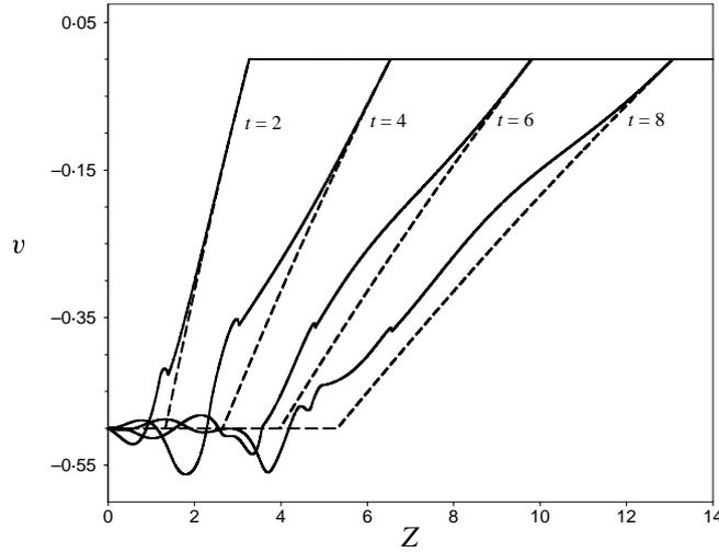
FIG. 6.  $v$  as a function of  $Z$  at various times for the Blatz–Ko model (2.19). The dashed lines represent the simplified solution obtained from the limiting case.  $L = 14$ ,  $v_0 = 0.5$ .
