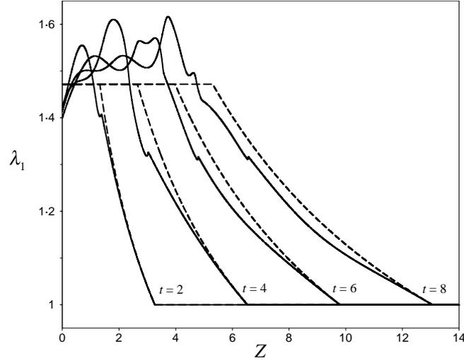
FIG. 5.  $\lambda_1$  as a function of  $Z$  at various times for the Blatz–Ko model (2.19). The dashed lines represent the simplified solution obtained from the limiting case.  $L = 14$ ,  $v_0 = 0.5$ .
