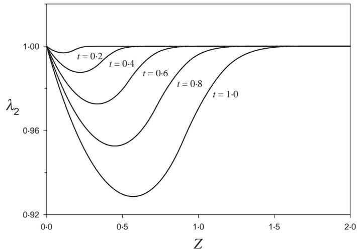
FIG. 8.  $\lambda_2$  as a function of  $Z$  at various times for the Blatz–Ko model (2.28).  $L = 2$ ,  $v_0 = 1$ .
