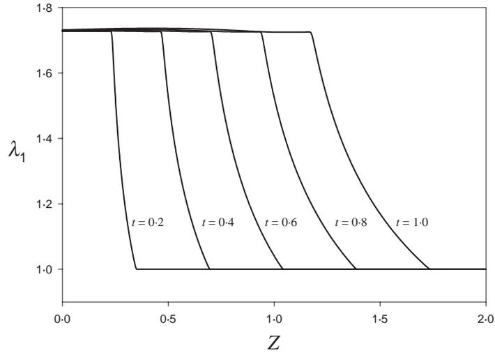
FIG. 7.  $\lambda_1$  as a function of  $Z$  at various times for the Blatz–Ko model (2.28).  $L = 2$ ,  $v_0 = 1$ .
