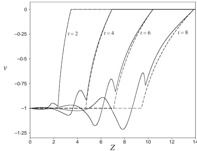
FIG. 12.  $v$  as a function of  $Z$  at various times for the Blatz–Ko model (2.28). The dashed lines represent the simplified solution obtained from the limiting case.  $L = 14$ ,  $v_0 = 1$ .
